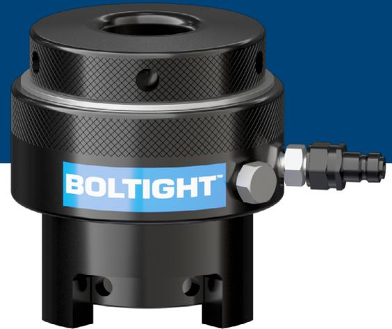
Because the force produced by the jack is applied directly to the end of the bolt, a tension equal to the load generated by the jack is developed in the shank of the bolt. With the jack applying the tension, it is possible to turn the nut with zero torque until its tight.
