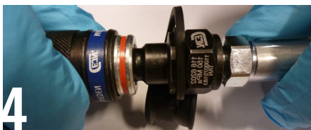
Check the red line is not visible – if red line is visible the connection is not safe to use
