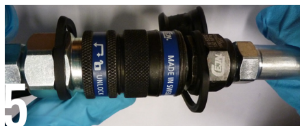
To close the safety locking sleeve (SLS) push the shroud forward to the back of the collar and rotate – release to lock
