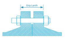
Always check that the tensioning force will not exceed 95% of the yield strength of the bolt material. If it does, the grip length of the bolt must be increased. Please contact your representative for advice on this.
